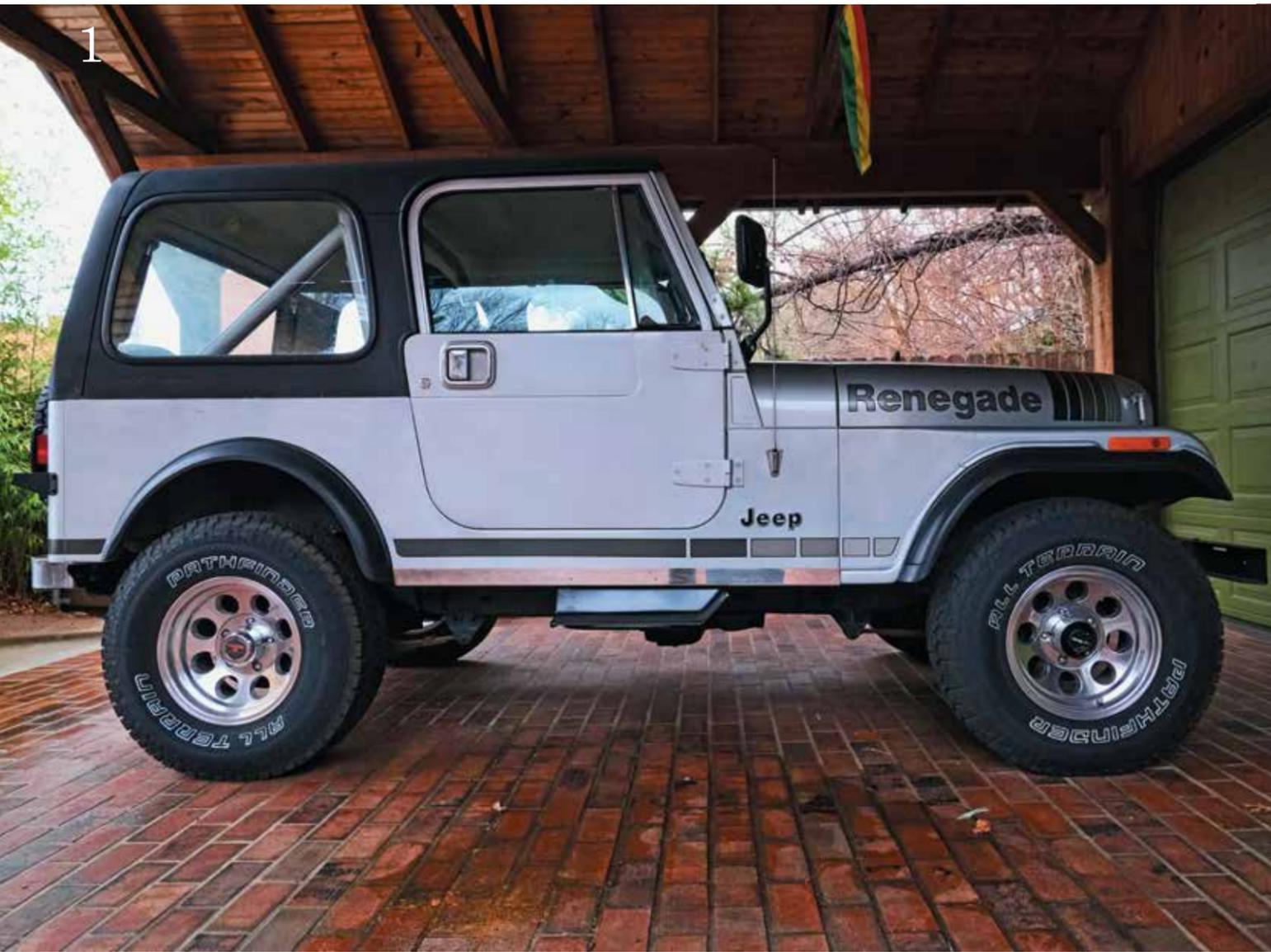
(1) Before replacing the springs, the original soft suspension sagged heavily in the front.
